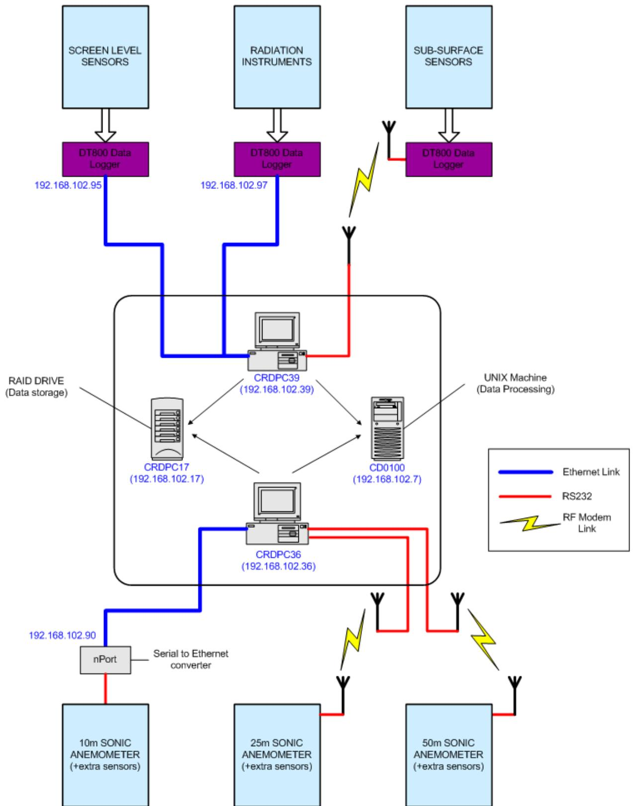
Figure 19: Logging schematic diagram.
