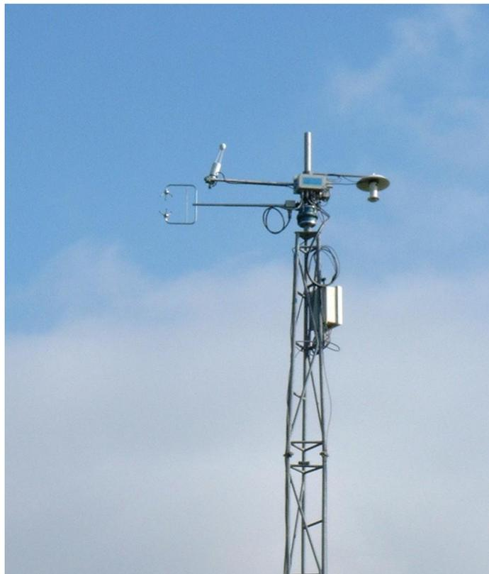
Figure 4: The *LI-COR* LI-7500 gas analyser co-located with a sonic anemometer, on the 10 m tower.
