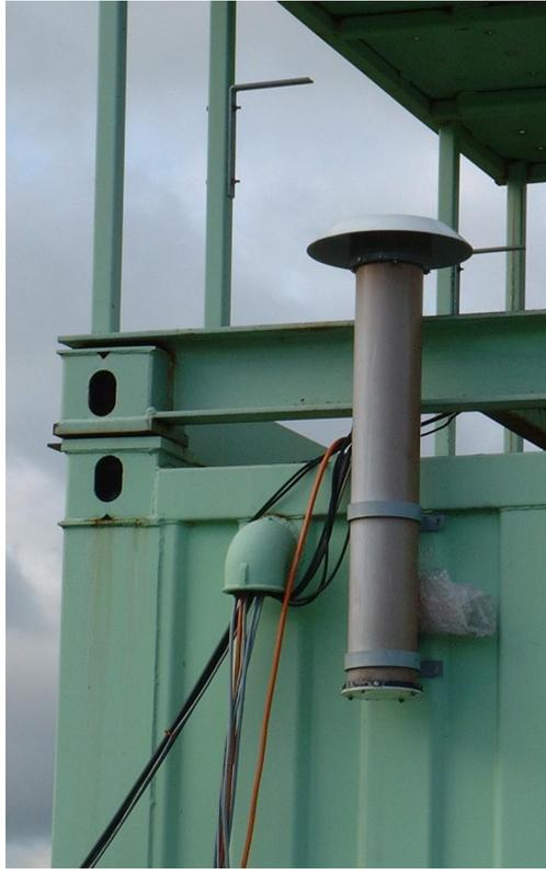
Figure 16: Nephelometer air inlet pipe outside hut.
