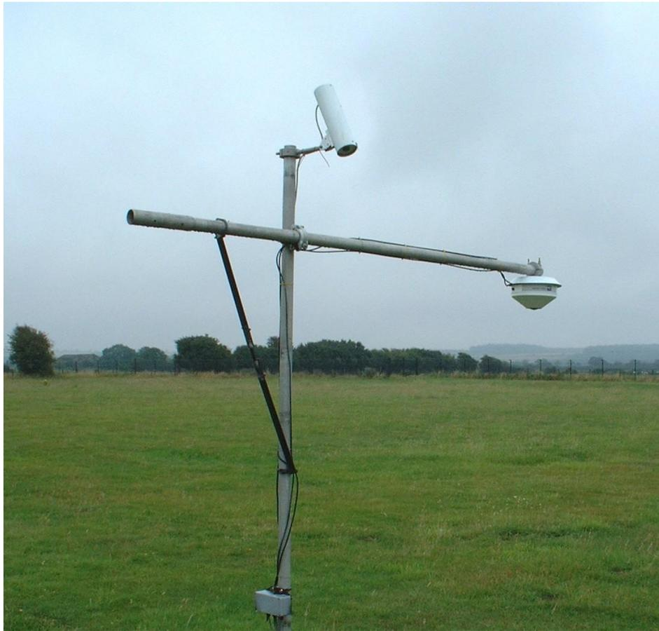
Figure 8: Downward-facing pyrgometer at end of boom, and *Heitronics* IRT pointing at the ground.
