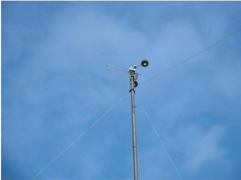
Figure 2: Ultrasonic anemometer mounted at the top of the 25 m mast. (Also present: temperature and humidity sensors inside aspirated screens.)
