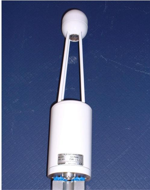
Figure 5: *LI-COR* LI-7500 gas analyser.
