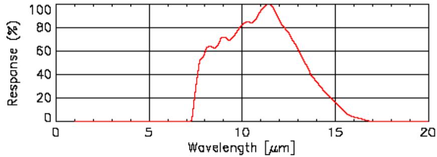
Figure 13: Spectral response curve of KT15.82D
