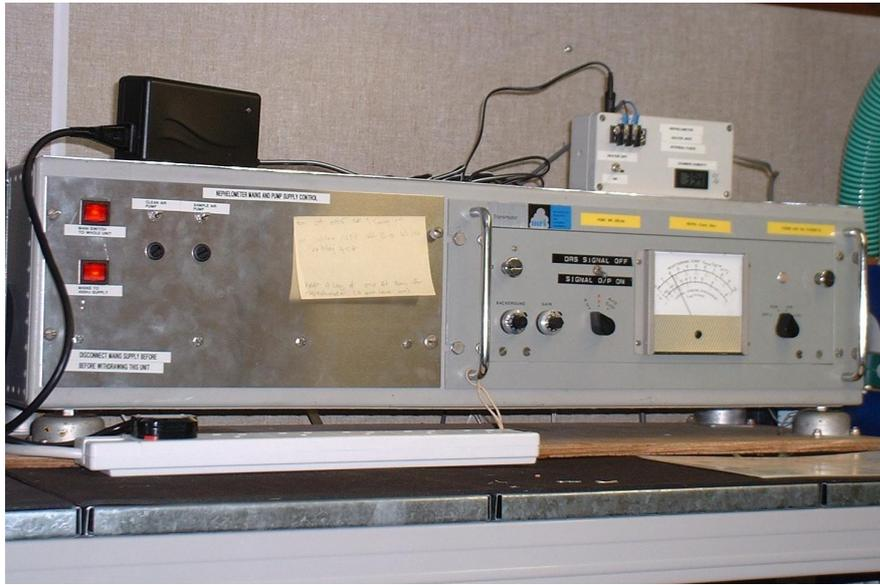
Figure 14: Nephelometer control unit
