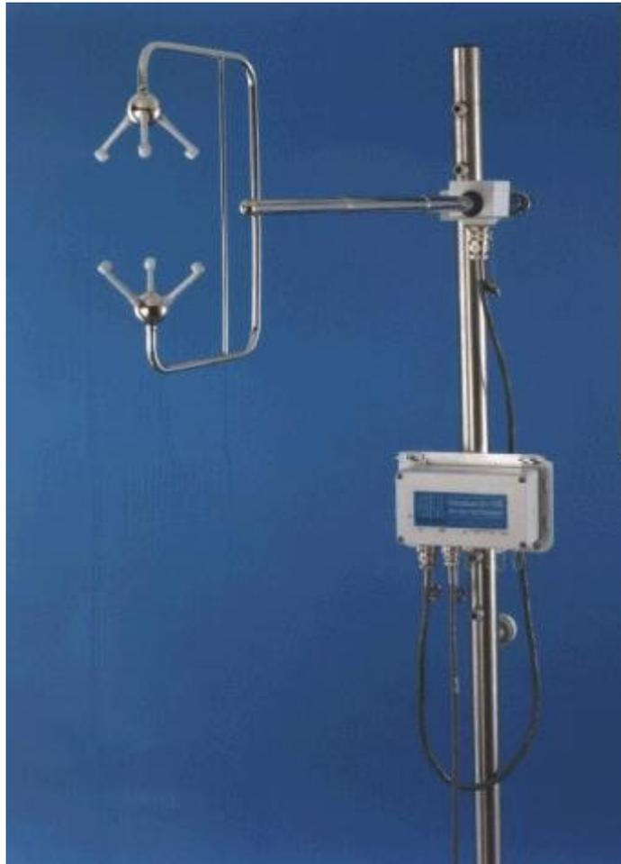
Figure 3: Gill HS ultrasonic anemometer
