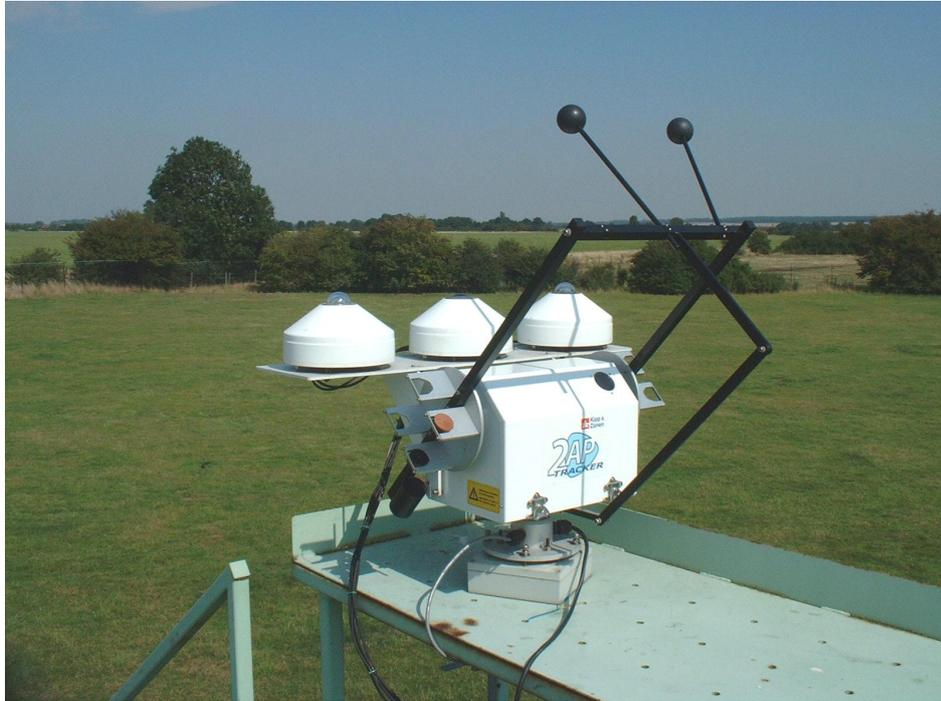
Figure 7: Radiometers mounted on a *Kipp & Zonen* solar tracker.
