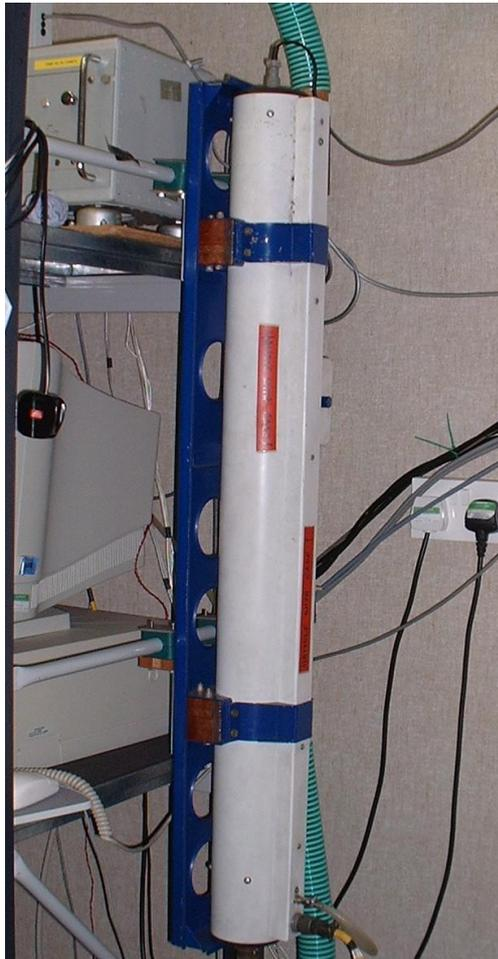
Figure 15: Nephelometer optical assembly
