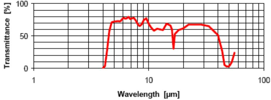
Figure 11: CG4 Transmittance characteristics graph, source *Kipp & Zonen CG4 manual*.
