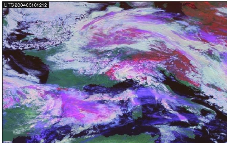
Figure 2 RGB image of Europe, made from SEVIRI channel 1 ( $0.64 \mu\text{m}$ ), channel 3 ( $1.6 \mu\text{m}$ ) and a combination of channels 4 ( $3.9 \mu\text{m}$ ), 9 ( $10.8 \mu\text{m}$ ) and 11 ( $13.4 \mu\text{m}$ ). The scene was acquired on March 10<sup>th</sup>, 2004, around 12:12 UTC
