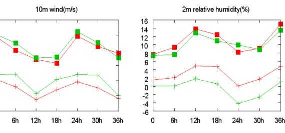
Figure 2. Biases (crosses) and RMS errors (rectangles) of surface parameters of HIRLAM ETA area (red) and ECMWF (green) in July 2006. 00 GMT forecasts are used to compute the statistics.
