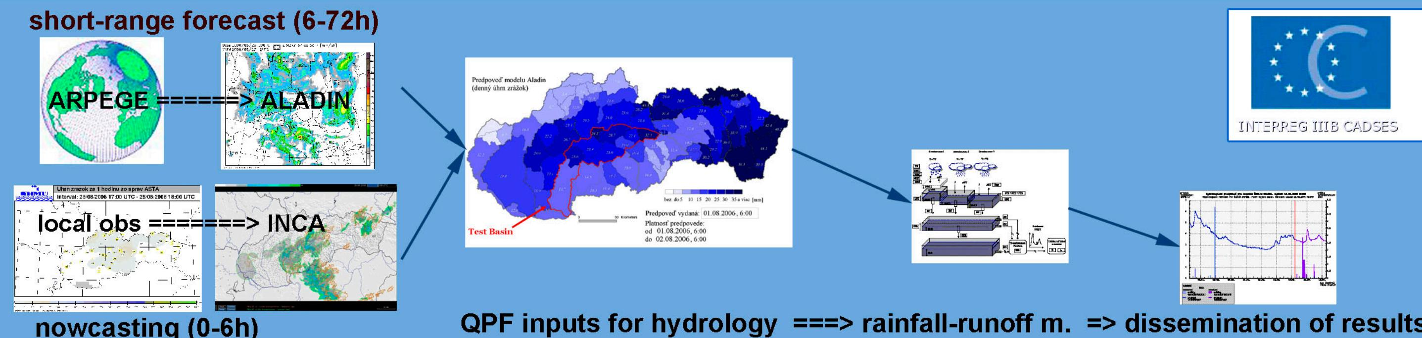
Aims at the consolidation of the flood forecasting and warning technological link at SHMU to complete the meteo-hydrological forecasting and warning cascade:
