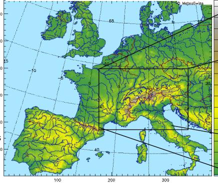
Figure 1: Operational domain of aLMo with a mesh size of  $\sim 7\text{km}$  showing the orography (maximum height at 3110m).
