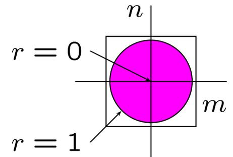
$$r_{m,n} = \sqrt{\left(\frac{m}{M}\right)^2 + \left(\frac{n}{N}\right)^2} = \frac{k}{k_{\text{max}}}$$
