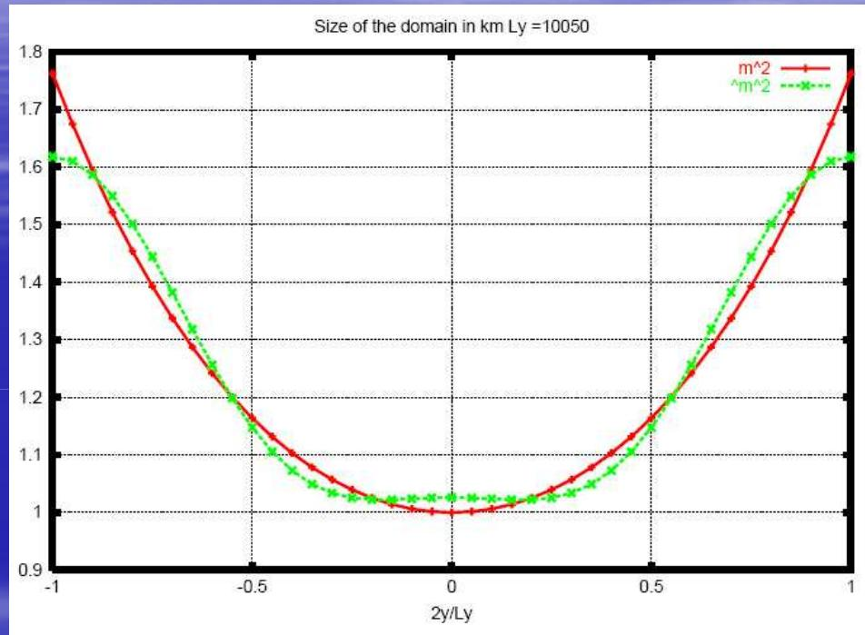
**Fourier estimation** of the square map factor with three coefficients ( $a_0$ ,  $a_1$  and  $a_2$ ) in comparison to the square **map factor real value**.  $L_y = 10.050\text{km}$
