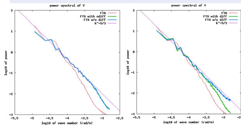
Fig.3 Spectra computed from ASUCA (left) and JMA-NHM(right). Spectrum at FT=0 (red), FT=9 w/o numerical diffusion (blue), FT=9 w/ numerical diffusion (green), and  $k^{-5/3}$  lines are displayed.
