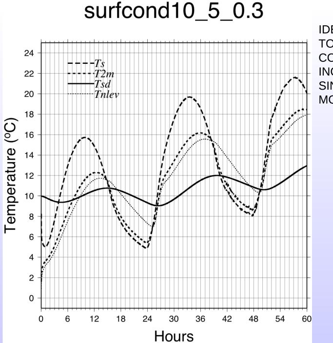
IDEALISED SENSITIVITY TO HEAT CONDUCTIVITY INCREASE. HIRLAM SINGLE COLUMN SOIL MODEL.
