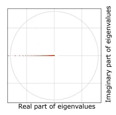
Eigenvalues of Laplacian operator (red dots) are pure real and negative – condition for stability of SI time stepping without nonlinear residual
