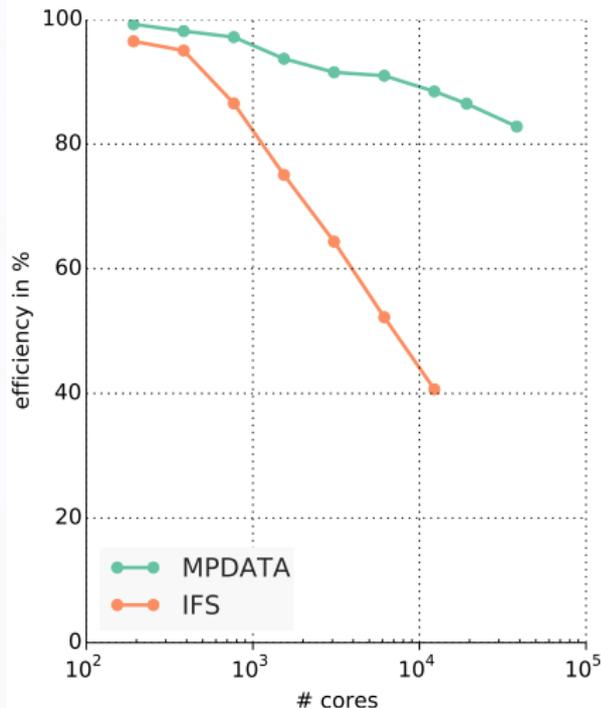
Scaling results obtained with 10km Reduced Gaussian mesh and 137 Levels.
