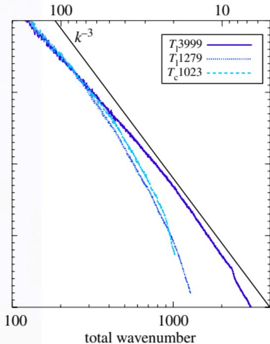
Comparison of global spectra after 5 days of simulation for the resolutions  $T_c1023$  and  $T_l1279$  at the lowest model level  $\sim 10$  m height (left) and at a mid-tropospheric model level  $\sim 500$  hPa (right)
