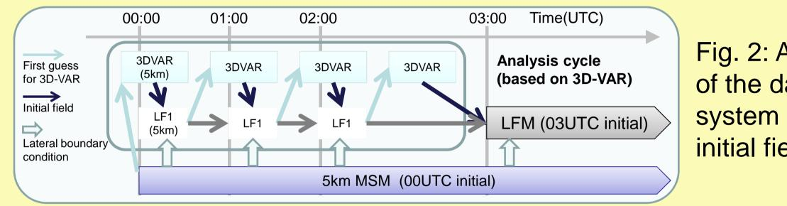
Fig. 2: A schematic diagram of the data assimilation system which provides an initial field for LFM.
