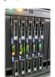
As a front-end fo the HPC machine, an high-availability virtualization system will be used, the IBM Blade Center. Each node is a Xeon X5650 with 6 cores at 2,67 GHz; 36 GB of RAM is also available. Linux (Ubuntu) and Windows will be used as OS. The system is also suitable for visualization, pre- and post-processing.
