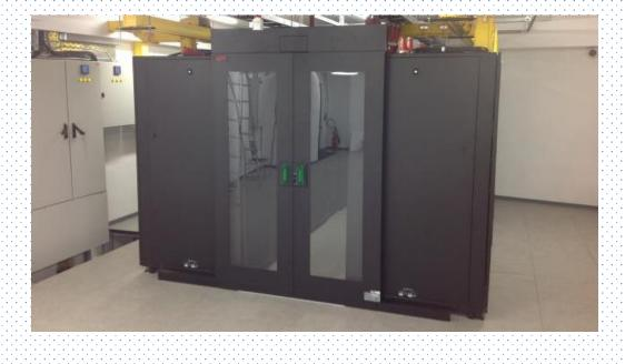
With 426 computational nodes, offers a total of over 8500 processing cores (CPU cores) interconnected network FDR Infiniband, an interface technology that offers low latency and high bandwidth. Additionally, it offers high performance storage, sized approximately 1 Petabyte, based on the IBM GPFS.
