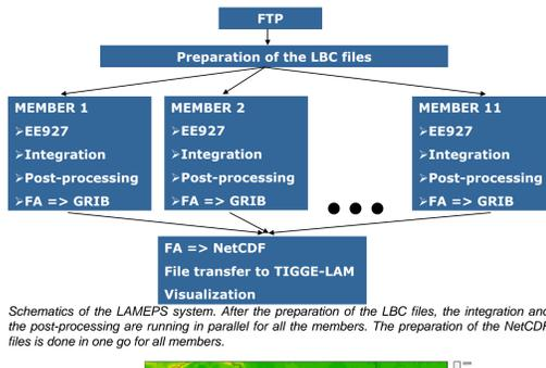
Schematics of the LAMEPS system. After the preparation of the LBC files, the integration and the post-processing are running in parallel for all the members. The preparation of the NetCDF files is done in one go for all members.
