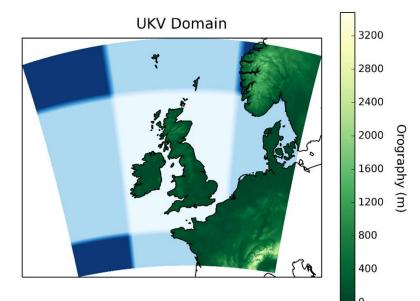
The UKV uses a rectangular grid in rotated lat-lon coordinates with variable spacing. The sea is coloured according to grid box area (with 4x4km boxes dark blue)
