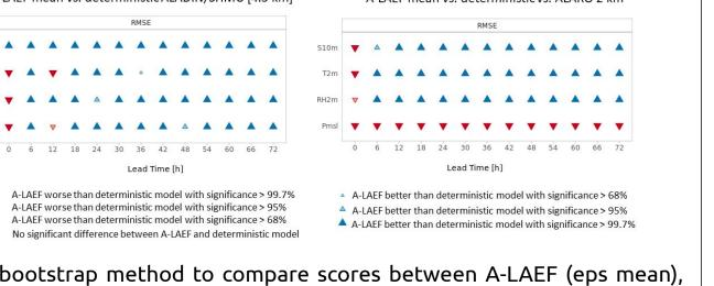
HARP bootstrap method to compare scores between A-LAEF (eps mean), ALADIN SHMÚ (operational) and ALARO 2 (test). Verification process is based on observation data from approximately 96 SHMÚ AWS stations.
