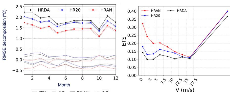
**Fig. 3.** RMSE decomposition (left) and ETS (right) for **HRDA**, **HR20** and **HRAN** wind speed predictions within the period 1. 1. 2022 - 31. 12. 2022. for 48 Croatian stations.
