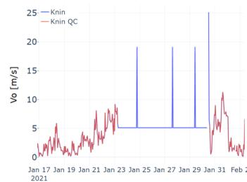
**Fig. 4.** The wind speed measured at the AWS Knin - an example of flagged unnatural steadiness of the wind with peaks (blue).
