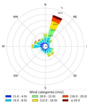
**Fig. 7.** The wind rose - measured at wind farm location (80 m; 5-month period).
