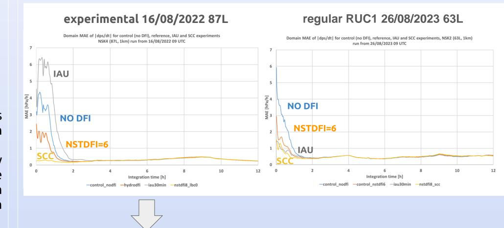
MAE of Pressure tendencies |dPs/dt| in hPa/h for the 16 August 2022 09 UTC experiment (cy46t1, 87L) between the 00 and 02 step of the run
